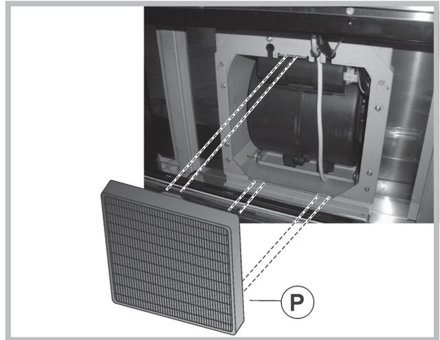
Replace the charcoal filter with one of the same type by carrying out the operations in reverse order.
