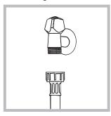
1. Connect the supply pipe by screwing it to a cold water tab using a 3/4 gas threaded connection (see figure). Before performing the connection, allow the water to run freely until it is perfectly clear.
