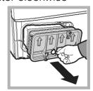
Clean the surface of the seals and replace, with the arrows pointing upwards making sure that the catches have been secured.
