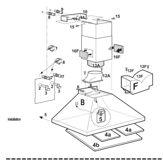
Warning! The position of the hook points (5 - Rectangular perforations) or the compulsory fastening points (8 - circular drill holes) may be inverted! Therefore check the back of the cooker hood in your possession to verify the position.
