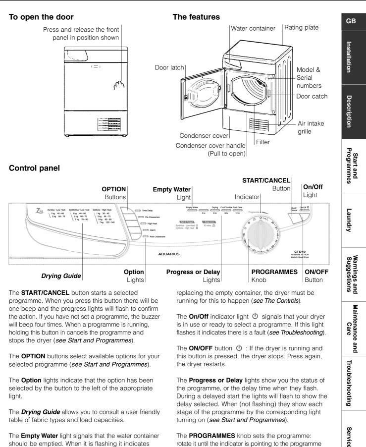
The Empty Water light signals that the water container should be emptied. When it is flashing it indicates that the container is full. The light will take a few seconds to go out after
