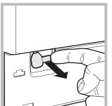
4. pull outwards using the tab as indicated in the figure, until the plastic tie-rod is freed from its stop position; pull downwards until you hear a "click", which indicates that the door is now unlocked.
