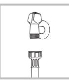
2. Connect the inlet hose by screwing it to a cold water tab using a 3/4 gas threaded connection (see figure).
