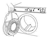
A very important part of your dryer is the fluff filter at the front edge of the drum. It's there to trap the particles of lint and fluff which are normally blown away when clothes are dried on the washing-line. if the filter is allowed to become blocked, the passage of warm air through the drum will be severely restricted. This means your clothes will take much longer than normal to dry and the cost of drying them will be increased. it may also damage your dryer.
