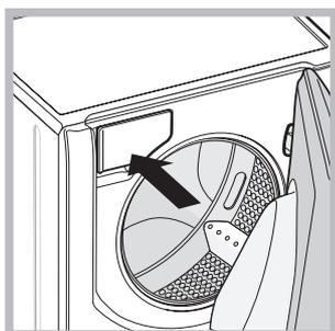
The detergent dispenser drawer is located inside the machine and can be accessed by opening the door. Refer to the chapter "Auto Dose System" for information on operation.
