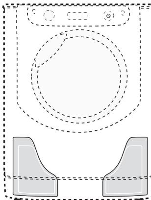
This washing machine is equipped with two tanks: one for liquid detergent (either concentrated or diluted) with a capacity of approx. 5.5 l and another for liquid fabric softener (either concentrated or diluted) with a capacity of approx. 3.5 l (see picture).
