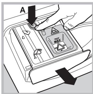
To fill the tanks with detergent and fabric softener, open the detergent dispenser drawer up to the first stop point then press lever (A) and open up to the second stop point, **ensuring that it is fully extracted**. Once the tanks have been filled (refer to "Filling the tanks"), the machine can run approx. 60
