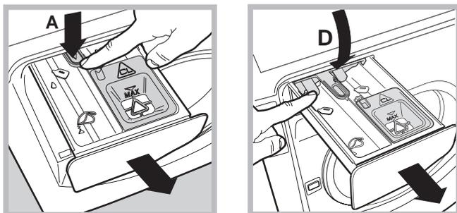
To pull out the dispenser drawer, open until the first stop point then press lever **A** to open completely; finally, press one of the levers **D** and pull the drawer outwards (see picture).
