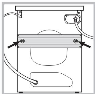
3. Remove the 2 protective screws and the rubber bush with the respective spacer, situated on the rear of the appliance (see also the installation leaflet). NB: The plastic spacers may fall down inside the machine once the bolt
